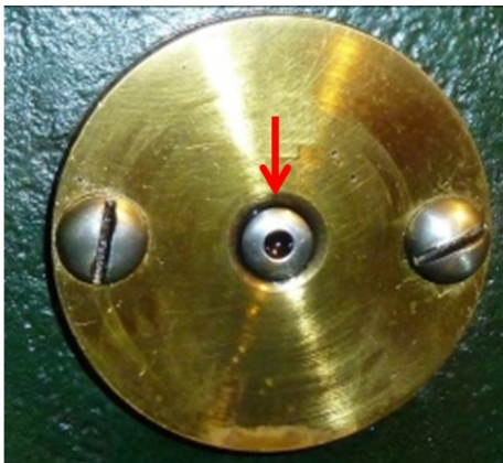
Close-up of bushing and where to apply oil
