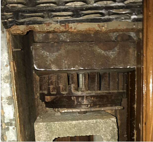
Striking weight resting on cinder block while a bit of cable is still on the striking drum
