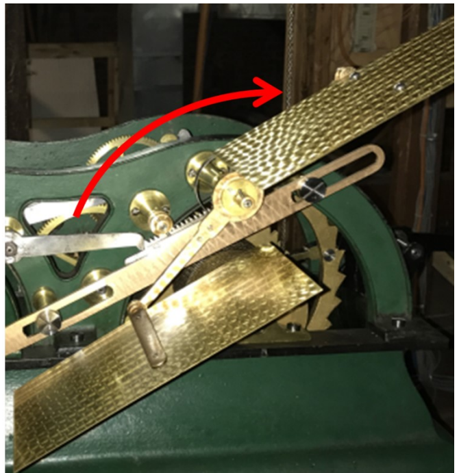
Rotate fan blades clockwise to complete prior strike
